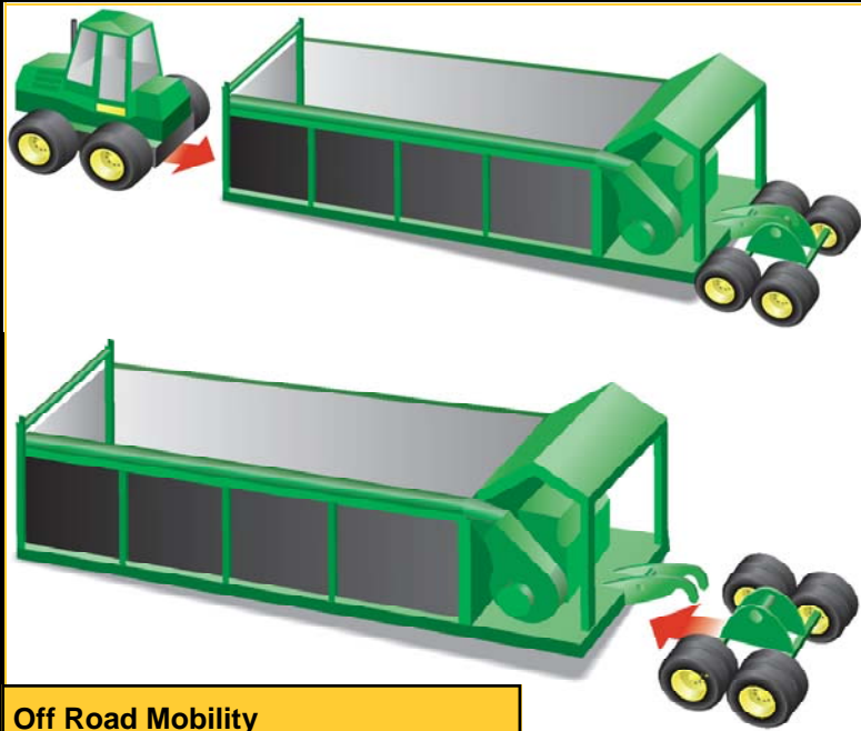
Off Road Mobility 8" of ground clearance Towable with tractor, loader, excavator, etc. Quick change, 10 minutes Aides with ash removal
