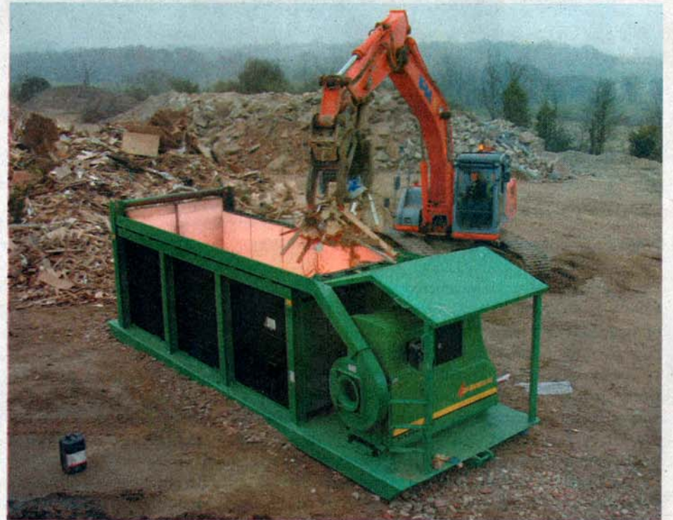
Burn box can handle timber residue, stumps, construction waste, and other debris. High velocity airflow creates an invisible curtain over fire and rotational turbulence within it.
