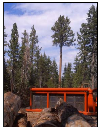
Air Burners S-116 in Full Operation: No Visible Smoke
