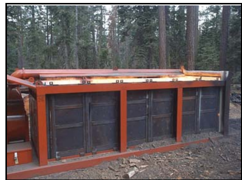
Air Burners S-116 in Full Operation (No Visible Smoke), Lake Tahoe, California
