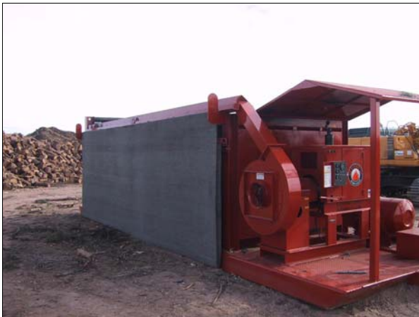
Ember Screen installed and hanging from support brackets
